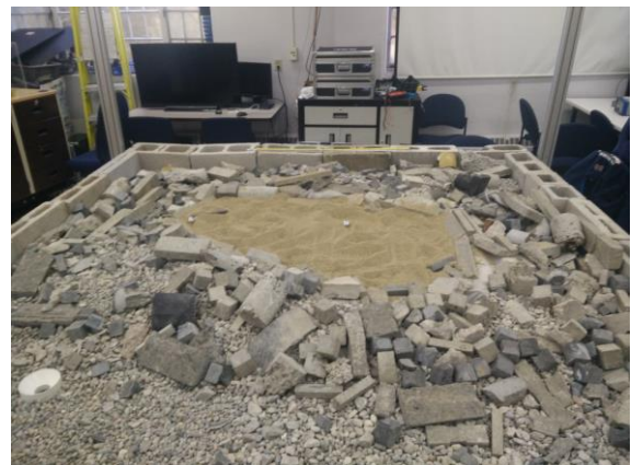
Figure 1: Arena layout for robot demonstration. Two spheres and an iron rod are the metal objects to be collected from the sand pit surrounded by a layer of rocks.
